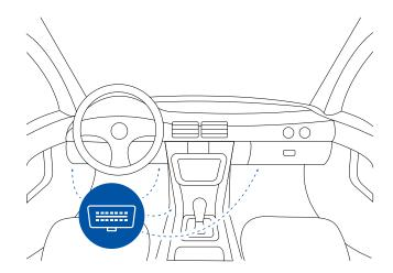
Most common OBDII connector locations.
