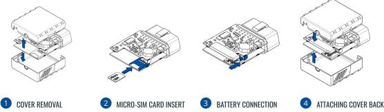
Gently remove FMB001 cover using plastic pry tool from both sides.
